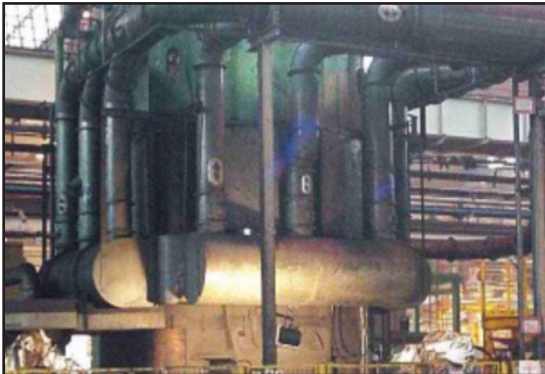
SCHLOEMANN 7700T Forging Press 900 mm ram, 450 bar, 50,000 cycle/month.
